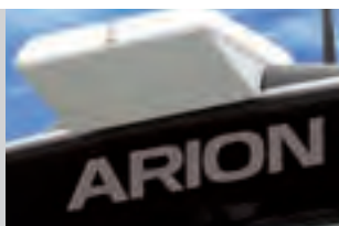
The OMNISTAR HP receiver for GPS signal and GPS reference signal.
