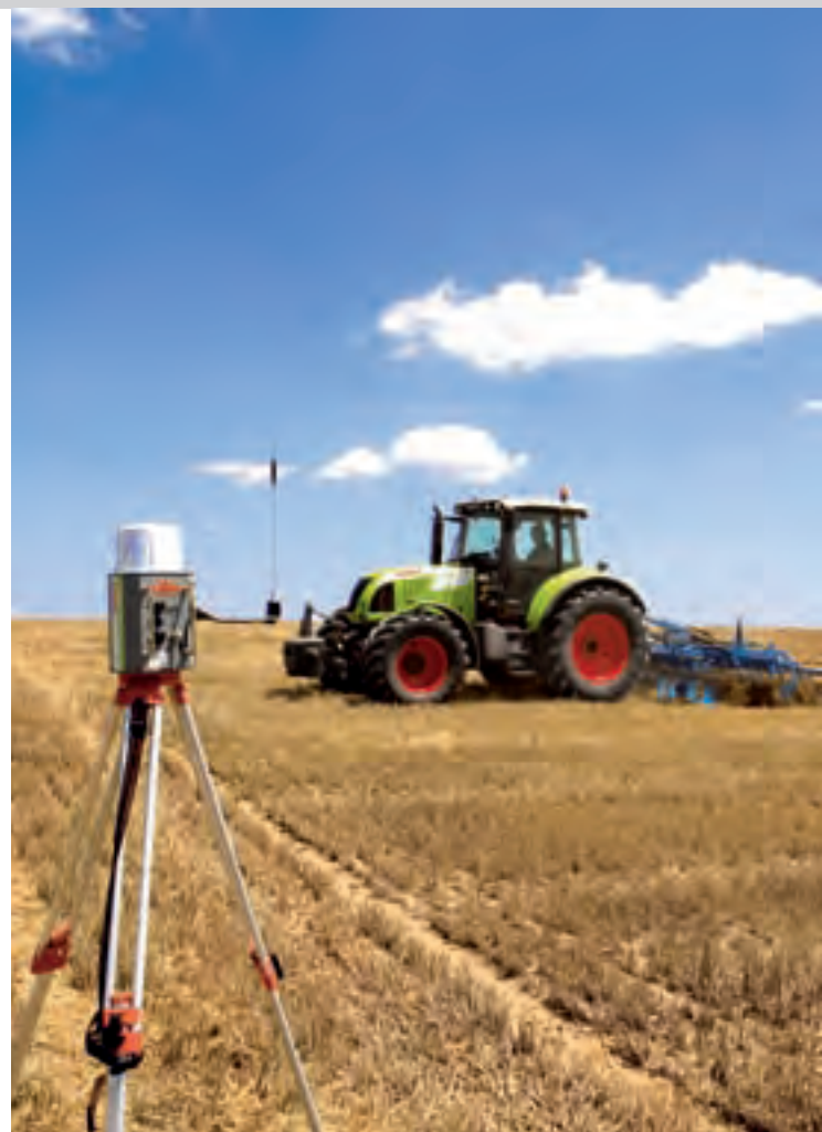
The GPS receiver on the BASELINE HD system. This includes an extra radio receiver for the reference signal.
