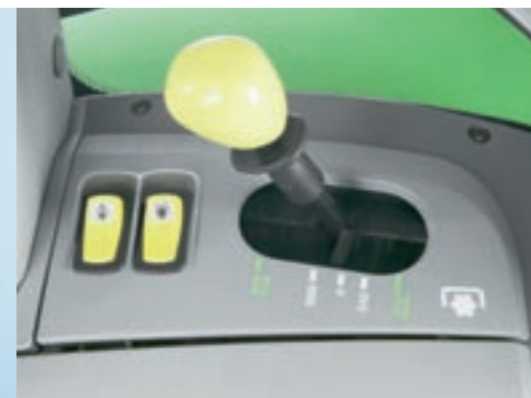
The standard four PTO speeds can be conveniently pre-selected.
