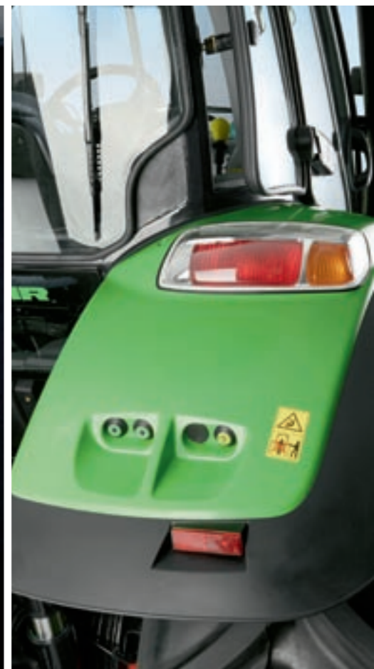
Powerlift and rear PTO can be safely operated from both rear mudguards.
