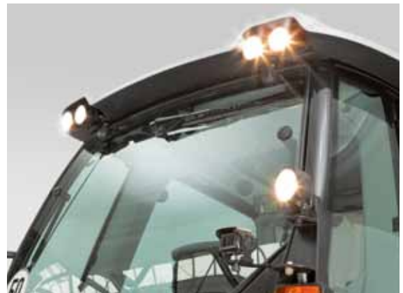
The rear of the Agrotron 410/420/430 is noticeable by its large visibility glass areas, high number of work lamps, and a reversing camera.
