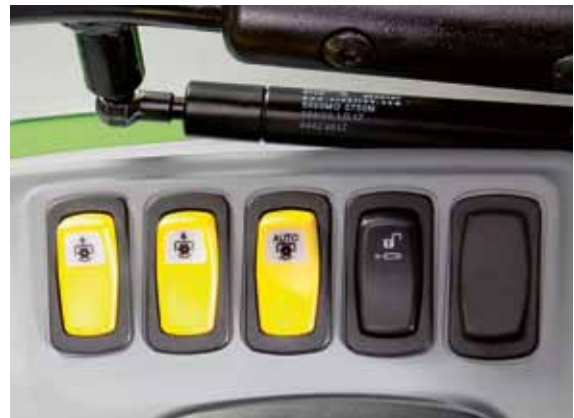
The standard auto power take-off disengages the PTO shaft whenever the rear hitch is operated.
