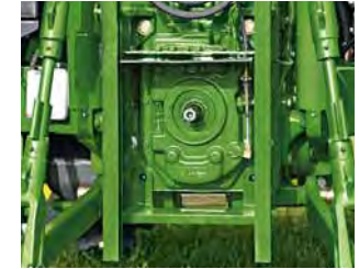
The PTO stub is located in a dry cavity.
