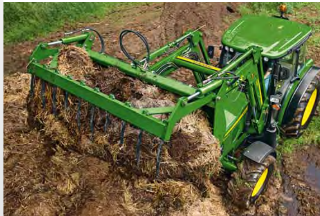
The front loader package has everything you need: mounting frames, hood protection, a mechanical 2-function joystick with diverter, an SCV block with pressure relief valve and a multi-coupler.
