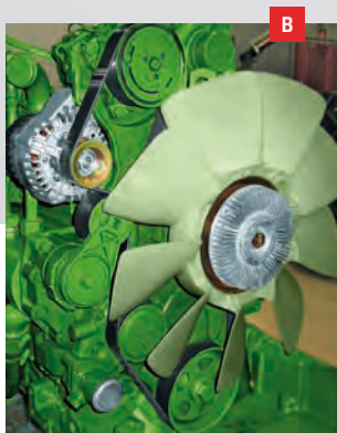
The viscous fan drive runs at reduced speed, leaving you more usable power.
