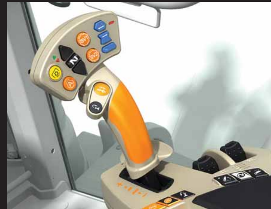
High spec MultiPad lever on the left-hand side of the Command Control Armrest and either fingertip or Multifunction joystick spool valve controls on the right-hand side of the armrest
