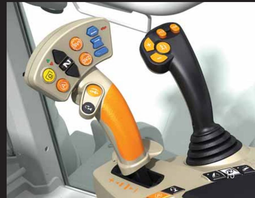
High spec MultiPad lever on the left-hand side of the Command Control Armrest and either fingertip or Multifunction joystick spool valve controls on the right-hand side of the armrest
