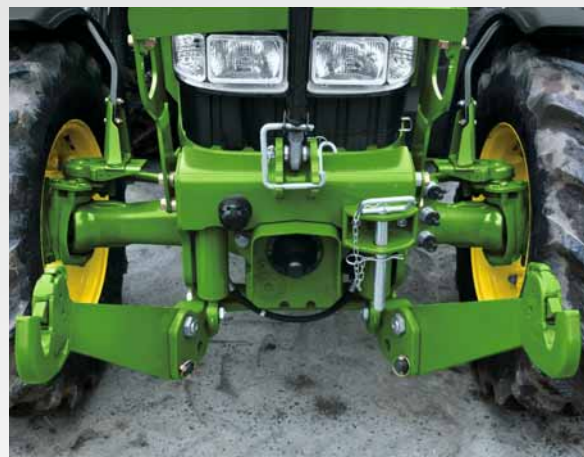
A fully integrated front hitch and PTO, ideal for front mowers or seed carts.
