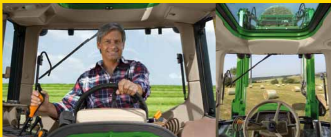
Optional roof hatch with glass makes it easy to see loads that are normally out of sight when working in tight, low buildings.
