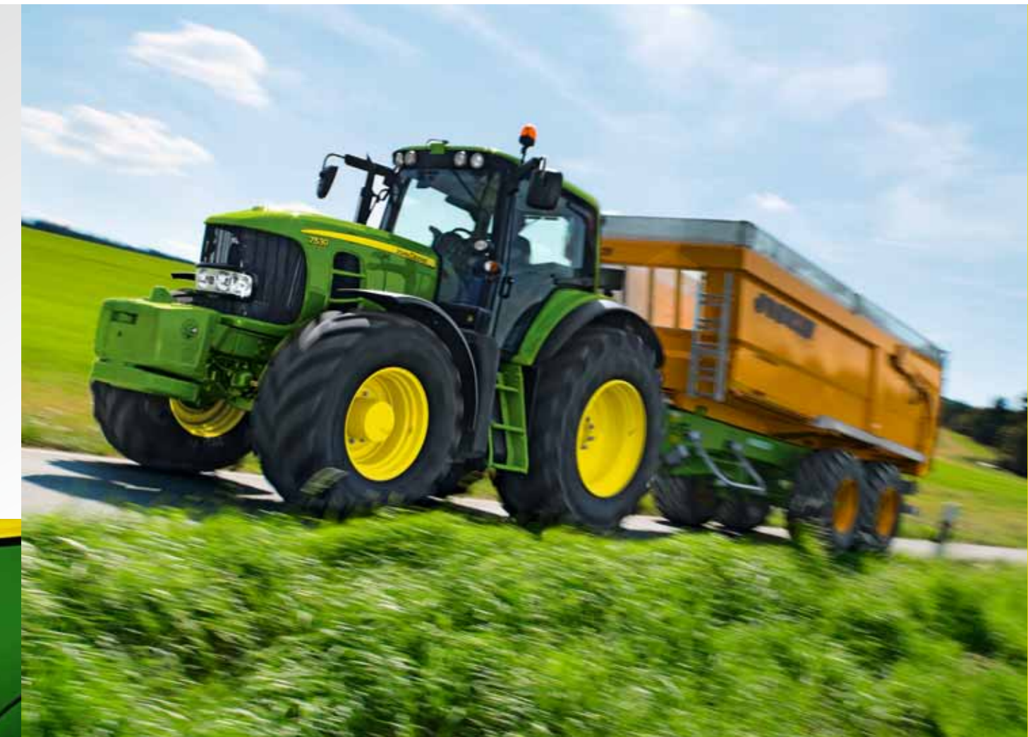
The all-new 7030 E Premium Series tractor is the first and only tractor with an electric generator to power auxiliaries such as engine cooling fan, air brake compressor, cab air conditioning compressor, providing a more efficient use of the engine performance. The E Premium line also provides 300 amp current for all other 12 V systems for both tractor and implements.
