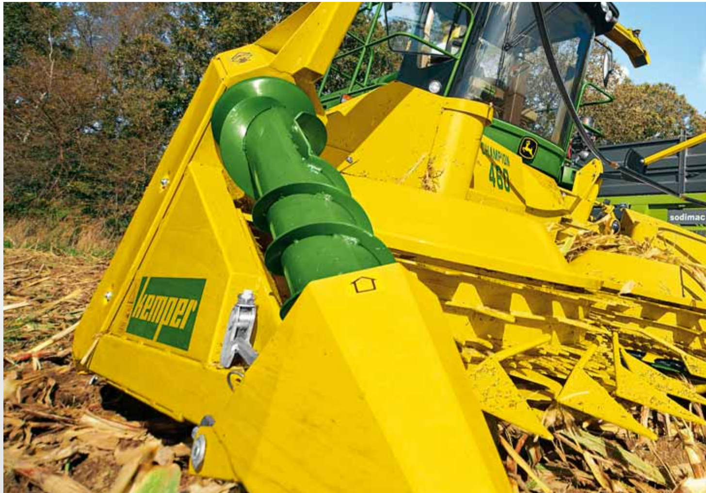
John Deere pioneered row independent cutting technology. This lets you cut maize in any direction, which is particularly important when harvesting laid crop.
