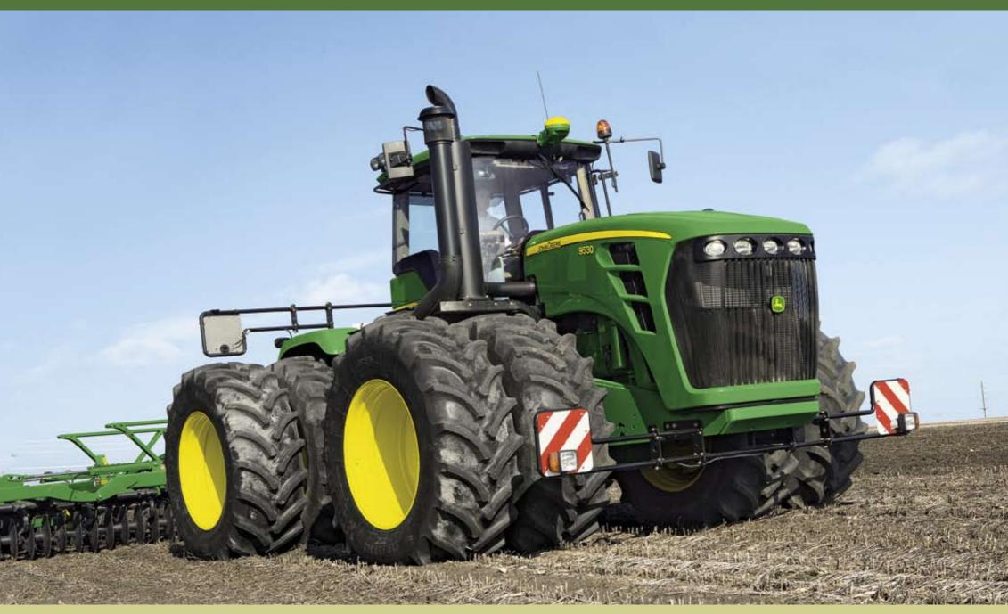
New 388 to 543 hp (289 to 405 kW) 9030 Series Tractors (97/68 EC)
