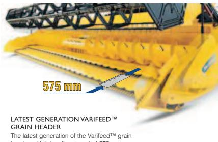
header which has floor travel of 575mm is available in three sizes: 7.62m (25ft). 9.15m (30ft) and 10.67m (35ft). All CR9000 elevation combines can be fitted with these headers. The rugged frame construction and the operational features including heavy-duty high speed knife drive, large auger diameter and extended reel tine reach guarantee an impressive cutting and feeding capacity, matching the throughput of the world's highest capacity combine range.
