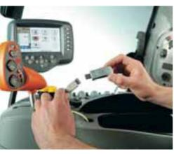
**Up to date information transfer** For the smooth exchange of data collected by the CX combine's yield sensor to the farm computer, a simple memory stick is used.
