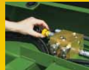
A twist of the bale density control knob adjusts the bale for crop and moisture changes.
