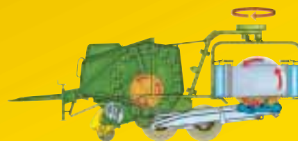
Twin wrapping arms quickly enclose the bale with film – thus eliminating air pockets which can cause spoilage.
