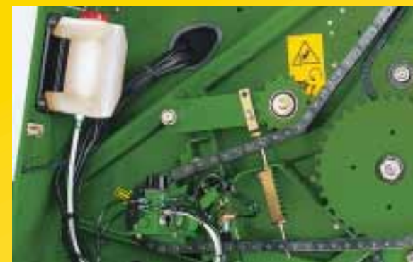
The optional automatic greasing system is controlled on the move.
