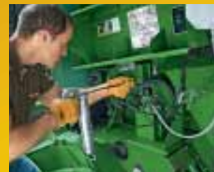
Central grease bank and automatic chain lubrication make servicing simple.
