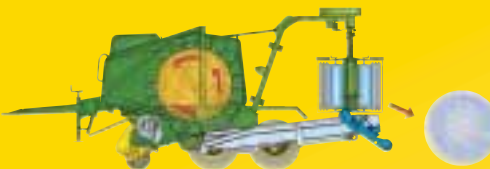
The transport table pivots down and carefully releases the bale.
