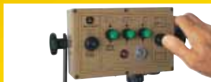
The ELC Plus monitor. The easy to learn and operate ELC Plus monitor offers fully automatic operations. Net and twine settings can be made without leaving the cab.
