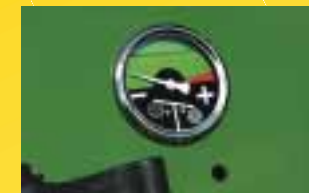
Adjust the bale density. The easy to access bale pressure gauge is conveniently located on the baler's front panel.
