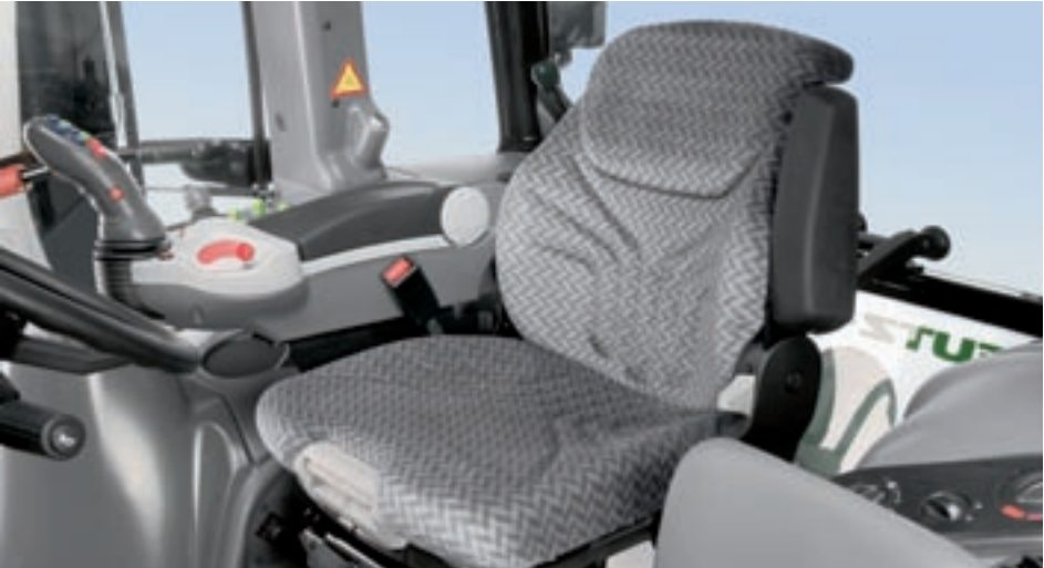
The air-suspended comfort seat offers more than 11 different functions to make it easy for the driver to find his individual, comfortable seating position.
