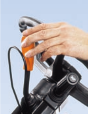
Changing the direction of travel without actuating the clutch: the standard Powershuttle .
