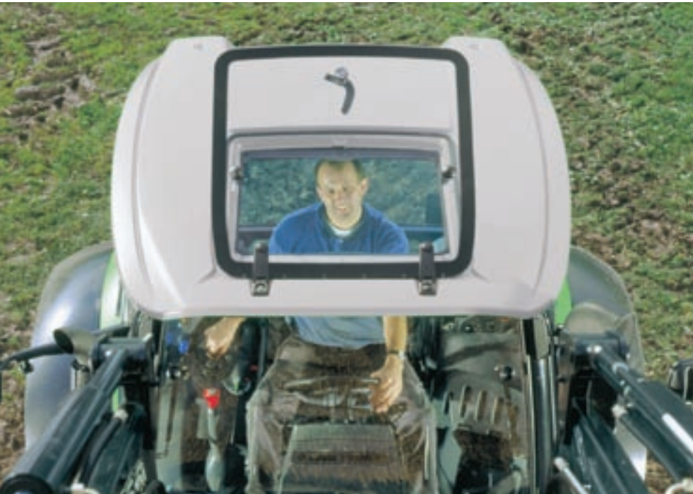
Unobstructed view to the top: The optional glass roof hatch provides an even higher degree of safety with a clear view of the raised DEUTZ-FAHR front loader.
