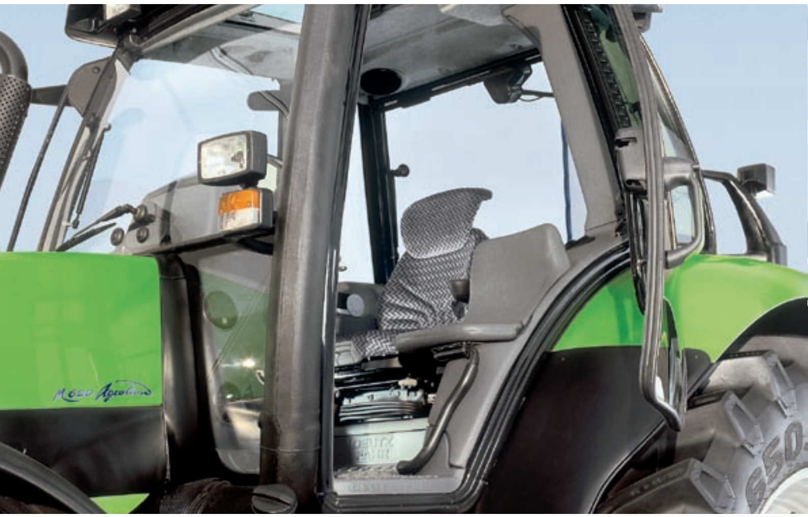
Easy mounting: Two full-length hand rails are mounted on each side.
