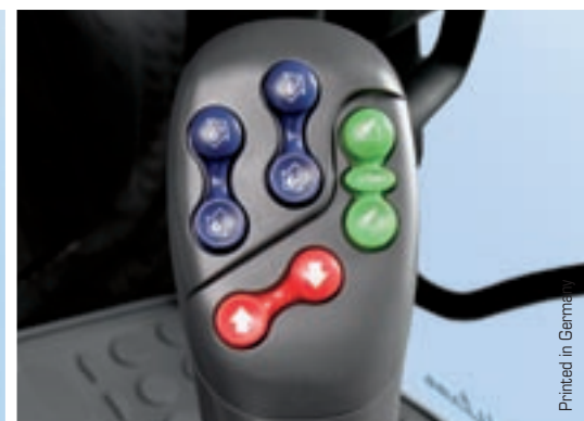
On the ProfiLine version the powerlift and remote valves 1+2 are operated directly with the PowerComS lever.
