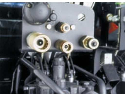
To order the Agrotor M can be fitted with Power-Beyond connectors for the direct connection of third-party devices.
