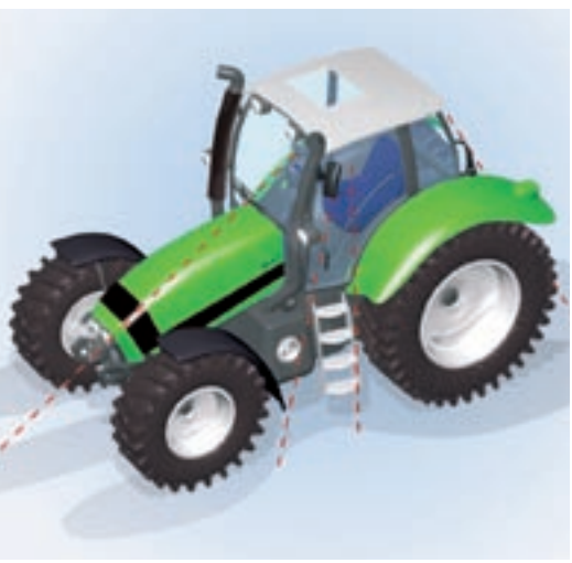
A cab design that still sets standards: With a panoramic view of 320° and cab glazing of 6,5 m 2 the spacious panoramic cab of the Agrotion is one of the largest available.
