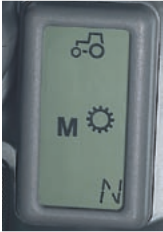
Everything in view: The central display of the Powershift stages in the A-strut.
