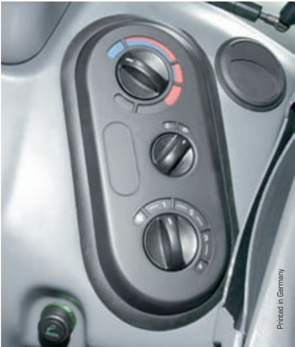
Automobile-standard air conditioning. The controls for the standard-feature air conditioning are integrated behind the instructor's seat.
