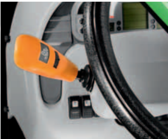
The hydraulic Powershuttle has five adjustable settings and makes the job of maneuvering much easier.
