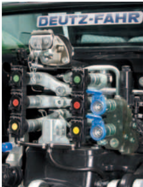
Easily accesible and clearly identified hydraulic connections. Up to four remote valves upon request.
