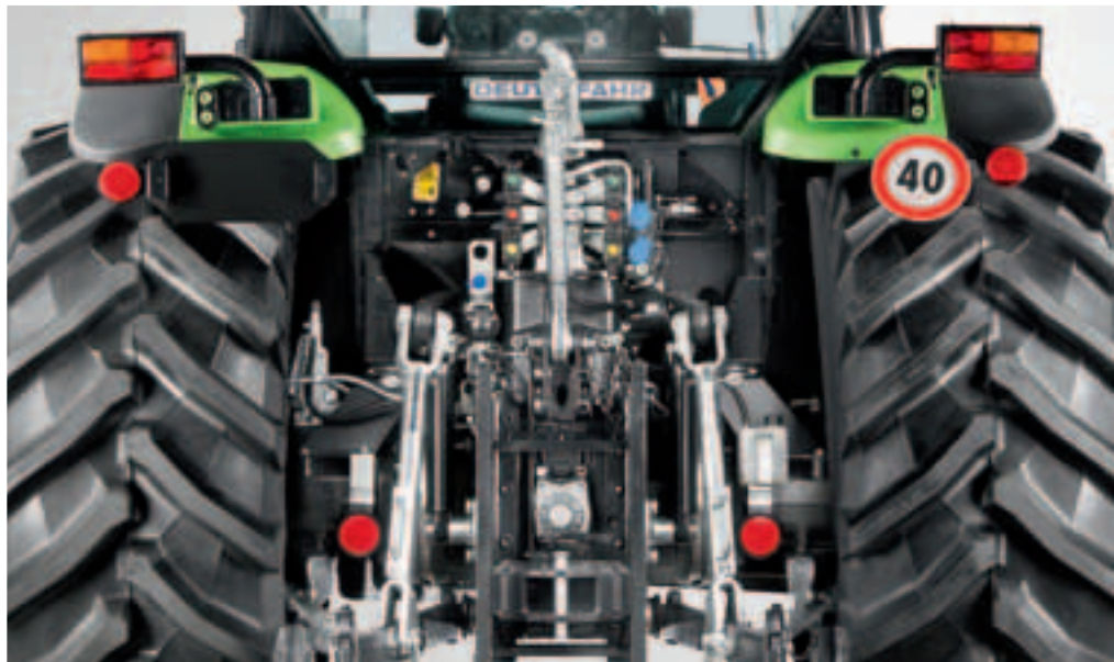
The powerful rear linkage with 5,300 kg lift capacity for operating the heaviest implements (6,200 kg with additional lifting rams for 430 model).
