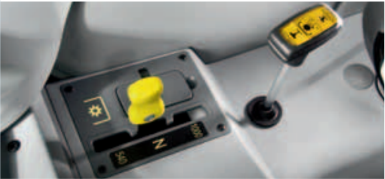
Comfortable in-cab pre-selection of four PTO speeds.
