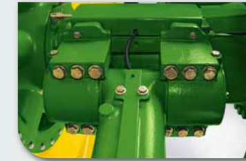
(5) Heavy duty reaction arm attaches to rear axle and pivots up and down.
