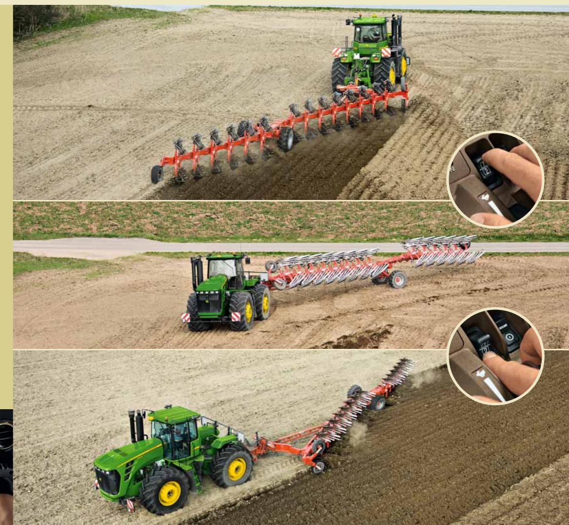
John Deere Implement Management System. You can simplify complicated turn sequences and even less experienced operators can become more productive in less time. Set IMS to simultaneously perform up to 20 tractor functions per switch (40 total) – push-button easy. IMS boosts efficiency and productivity plus it reduces operator fatigue.
