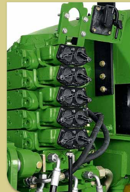
When greater hydraulic capacity is needed up to six SCV remotes are available as a field-installed option.
