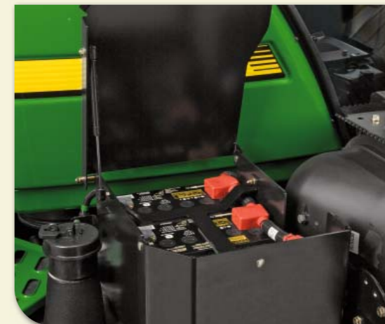
Flip-up battery cover features a gas strut to hold it up during periodic inspections or annual service.
