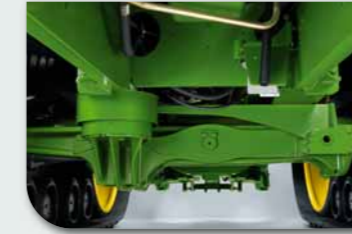
(1) Massive centre pin provides support for, and allows for the swing arm and walking beam to pivot.
