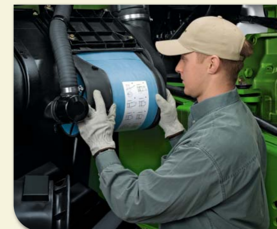
Annual air filter replacements are simple for all 9030 Series tractors. Filters can be conveniently reached while standing on the ground.
