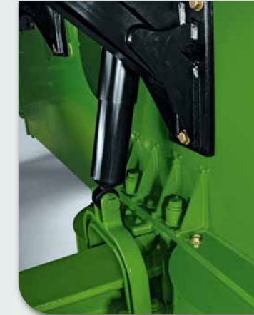
(4) Heavy duty shock absorber provides additional cushion as the walking beam travels vertically.
