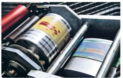
The printing units are based on dry offset technology and print the products at a speed of up to 300 units/min.
